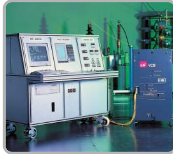
Characteristics Test / VCB Characteristics Test
